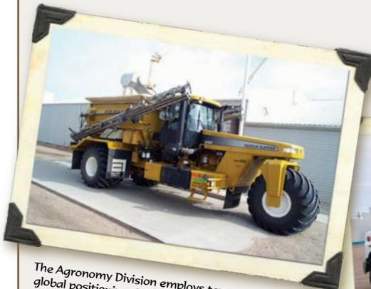
The Agronomy Division employs terrogators, with global positioning data and soil sampling results, to apply precision fertilizers, so the producer only pays for the fertilizer that is needed.
